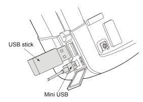
Figure 30. Test Tool USB Connections
