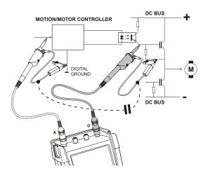
Figure 36. Parasitic capacitance between analog and digital reference
