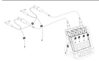
Figure 34. Parasitic capacitance between probes, instrument and environment
