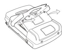
Figure 43. Removing the Battery Cover
