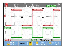
Figure 21. Time Measurement with Cursors
