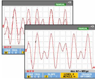
Figure 26. N-Cycle triggering
