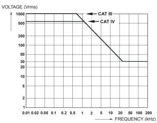
Figure 47. Safe Handling: Max. Voltage Between Scope References, and Between Scope References and earth ground.
