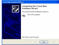
4 After completing the first step the New Hardware Wizard will start again to install the USB Serial Port Driver.
