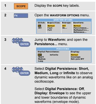
Select **Display: Dot-join: Off** to display measured samples only. Dot join off may be useful when measuring for example modulated signals or video signals.
