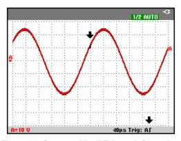
Figure 23. Screen with all Trigger Information
