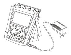
Figure 41. Charging the Batteries
