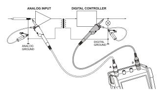
Figure 37. Correct connection of reference leads
