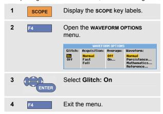
You can use this function to display events (glitches or other asynchronous waveforms) of 8 ns (8 nanoseconds, due to ADC's with 125 MS/s sampling speed) or wider, or you can display HF modulated waveforms.
