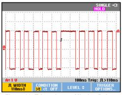
Figure 29. Triggering on Missing Pulses
