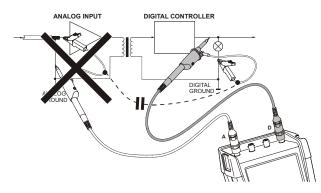
Figure 38. Wrong connection of reference leads
