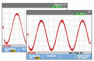
Figure 11. Smoothing a Waveform
