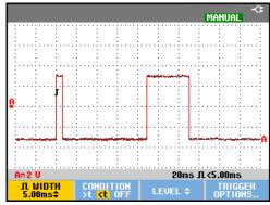
Figure 28. Triggering on Narrow Glitches
