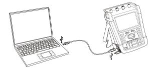
Figure 31. Connecting a Computer
