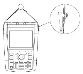
Figure 40. Fixing the Hangstrap
