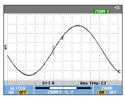
Figure 19. Zooming in a Waveform
