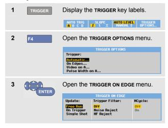
When **Free Run** is selected, the test tool updates the screen even if there are no triggers. A trace always appears on the screen.
